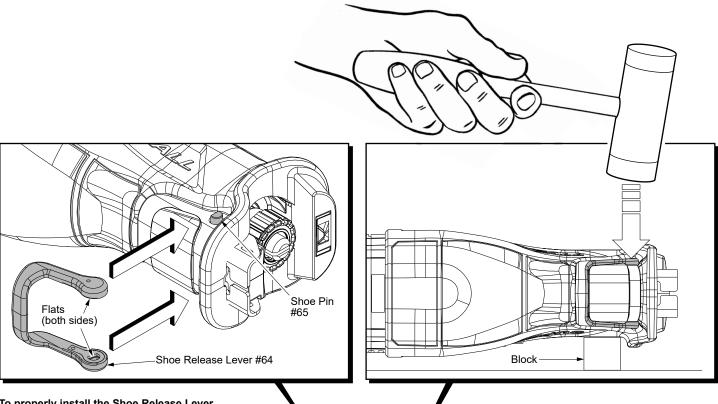
To properly install the Shoe Release Lever #64 onto the Shoe Pin #65 do the following:
